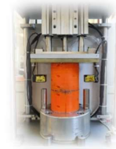
Thermal Impedance ASTM D5470-17 (IMS laminates characterization)
